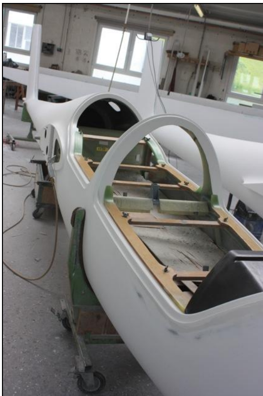
Here is the first preview of our new ASK21 VH-GVA under manufacture at the Alexander Schleicher factory in Germany. Photo: Schleicher's
